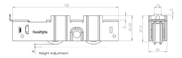
The brand new CA03 Heavy Duty Roller is specially designed to meet the current landscape of modern architectural accessories demands. The roller is fitted with the innovative TWIRO wheels, with double row bearing technology that offers effortless sliding action as well an excellent life span.
